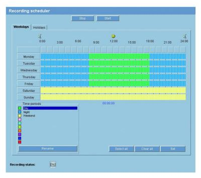
In the recording scheduler you can assign weekdays and times to the recording profiles you have created during which images from the camera should be recorded in the event of an alarm.
